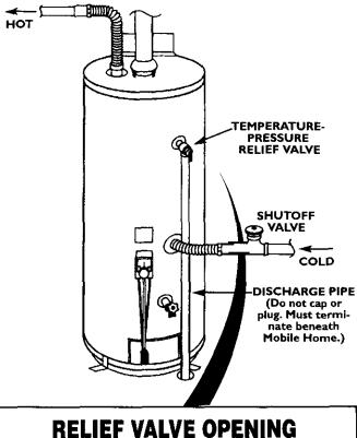
THIS WATER HEATER IS PROVIDED WITH A COMBINATION TEMPER-ATURE-PRESSURE RELIEF VALVE. FOR SAFE OPERATION OF THE
